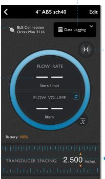
Indicates the strength of ultrasound within the pipe.
