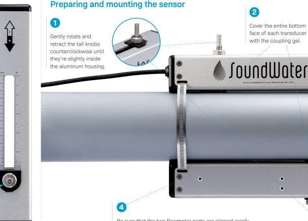
Be sure that the two flowmeter parts are aligned axially.
